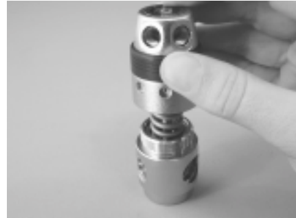
Figure 28. Installing piston assembly
