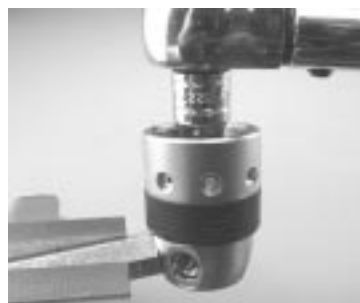
Figure 21. Torque retainer to 20 foot-pounds
