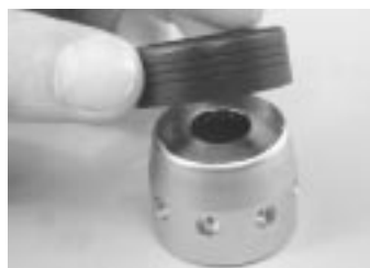
Figure 18. Install spacer onto tapered side of piston chamber
