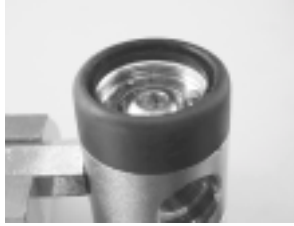
Figure 34. Install rubber cap
