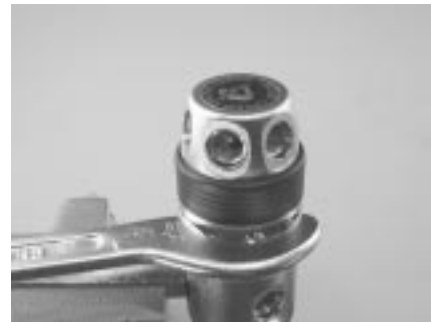
Figure 29. Tighten piston chamber with side spanner wrench
