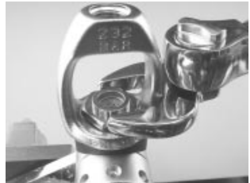
Figure 41. Torque inlet fitting to 20 foot-pounds
