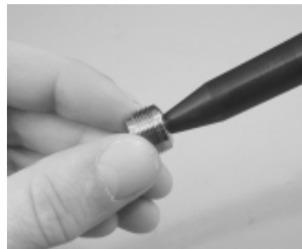
Figure 11. Blow HP seat with air nozzle
