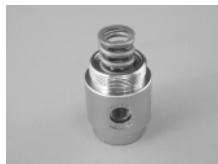
Figure 25. Install main spring
