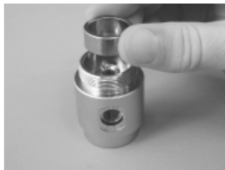
Figure 24. Install spring support
