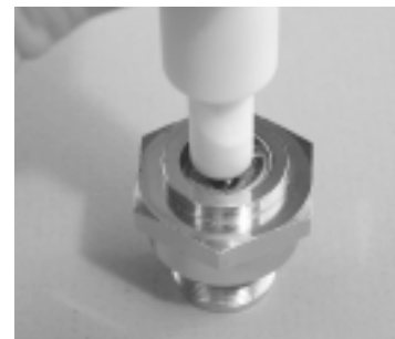
Figure 39. Use a dowel to ensure retaining clip is securely in place
