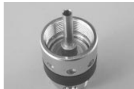
Figure 26. Press piston into piston chamber
