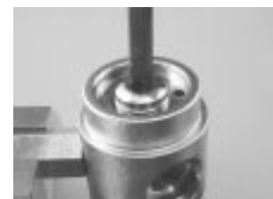
Figure 32. Install HP plug with 6mm hex wrench
