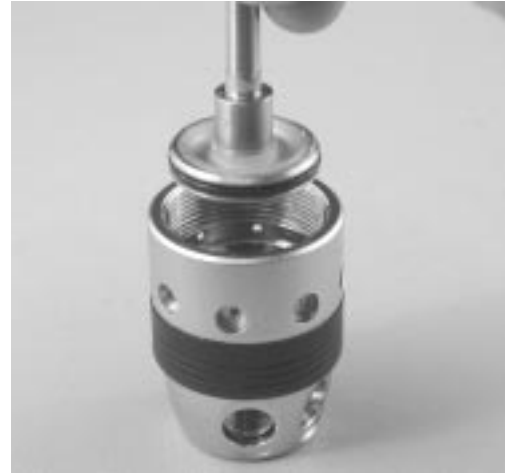
Figure 4. Remove piston from chamber
