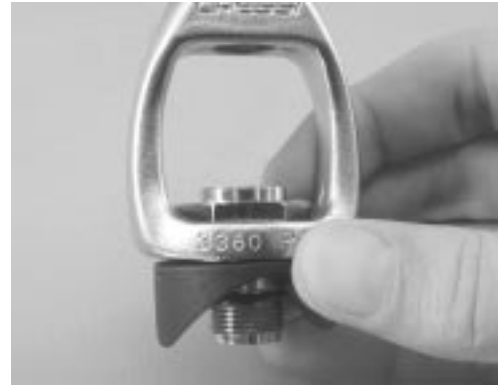
Figure 40. Pass inlet fitting through yoke and spacer
