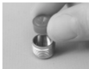
Figure 31. Install HP seat with conical side facing out
