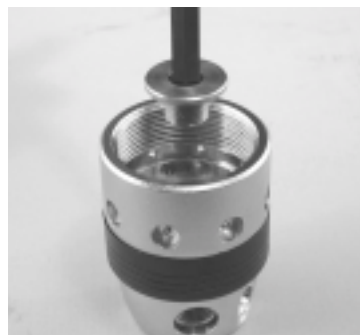
Figure 20. Install retainer with 6mm hex wrench
